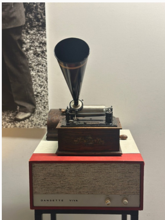
Early cylinder phonograph—a late 19th–early 20th century device used to record and play back sound on wax cylinders.
